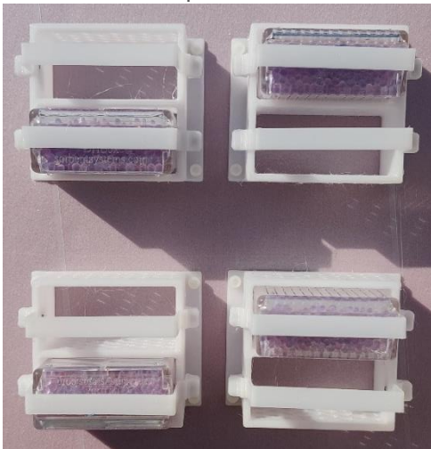
Figure 5. Installed DriBox desiccant on the back of the ICI Camera Enclosure door.
