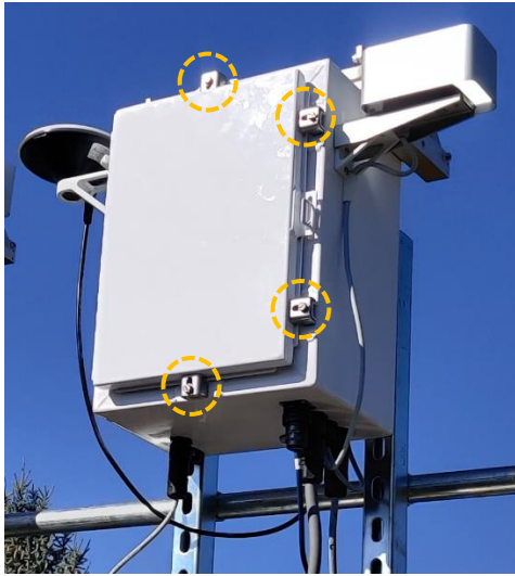
Figure 4. Photo of the Camera Enclosure front. The four retaining latches around the door are identified by dashed orange circles.
