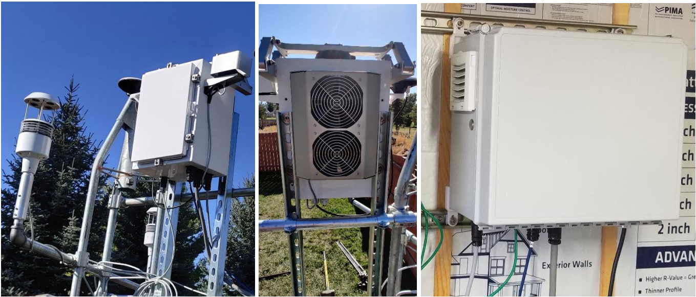
Figure 1. Front of ICI mounting with weather sensor option (left) rear of ICI Camera Enclosure (middle) Power Enclosure (right)
